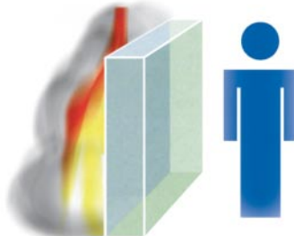
against flame, hot gases & smoke as well as a reduced surface temperature
